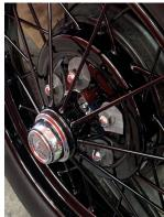
Moving along I scrounged up an old inner tube I've been using for various uses. I cut 10 pieces for both wheels with the center cut out to slip over the lug nuts9+9, they don't have to be perfect just enough to keep the lug wrench from touching the wheel and chipping the paint off. I also put some shrink tubing on the end of my lug wrench just in case I accidently bump a spoke. You can substitute the shrink tubing with a piece of hose taped over the end.
